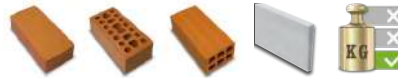
ladrillo macizo solid brick semimacizo semi-solid brick ladrillo hueco hollow brick yeso laminado plasterboard
